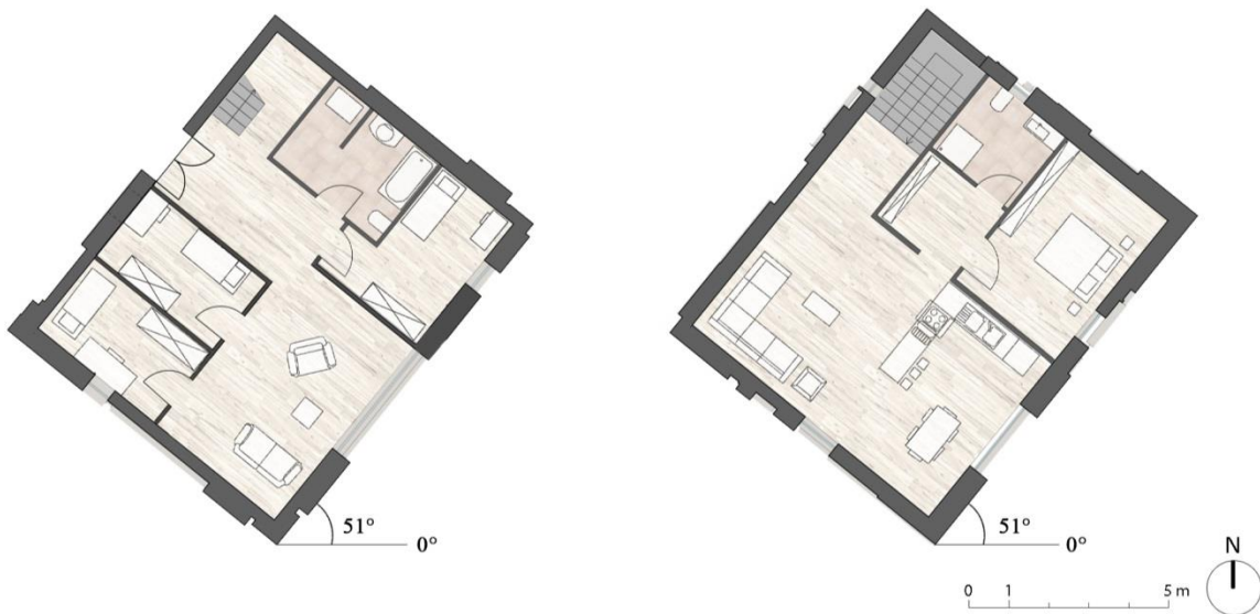
16 17 Figure 5. Stage 2 – Optimized Base Case : the ground floor (left) and the first floor (right) with the optimized orientation and the new inner 18 distribution of the spaces.
