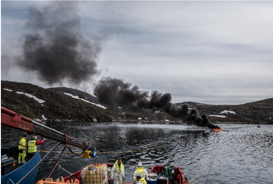
Figure 17: In situ burning experiment in Greenland 2017 (H2020 Project GRACE) with IFO180
