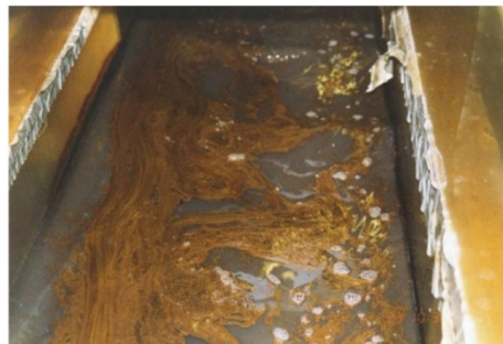
C) 30 min after the first application: approx.. 50% of the oil dispersed. Viscosity: 16570 cP (18% water)
