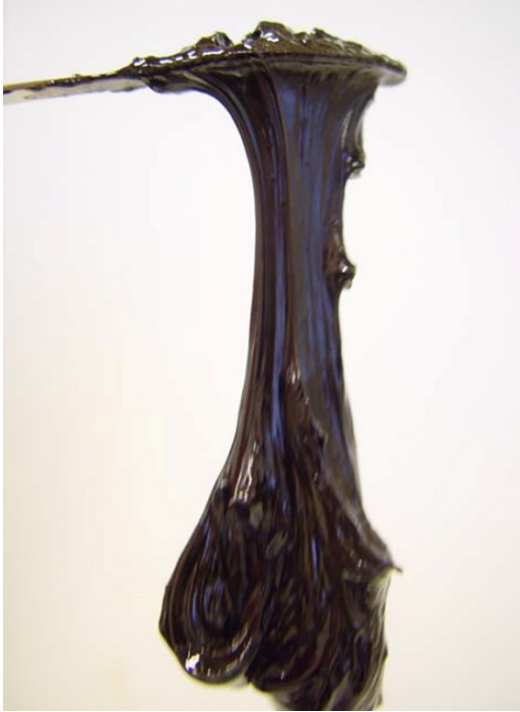
Figure 6: Example of Prestige oil after 61 days of weathering at sea. The oil was highly viscous, stiff and solid
