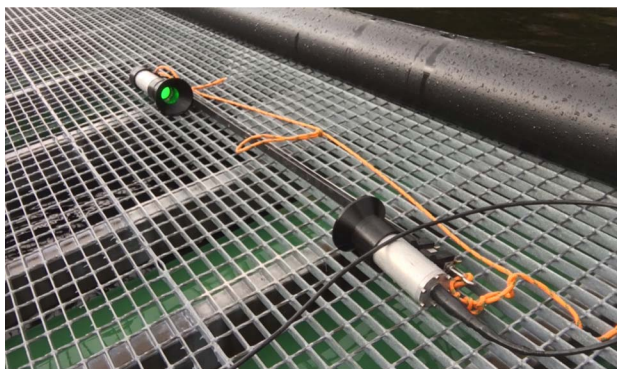
Fig. 14. Attenuation measurement instrument. The blinking green light source can be seen in the upper left corner, while the camera is located in the lower right corner. They are mounted 0.95 m from each other.
