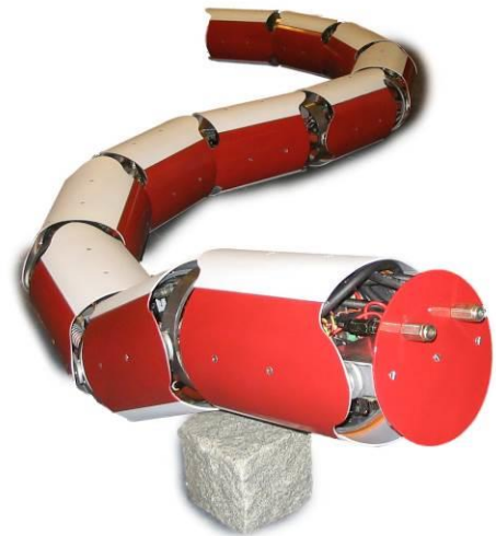
Figure 1: Anna Konda - a water hydraulic snake robot - for many years the world's largests snake robot [2].
