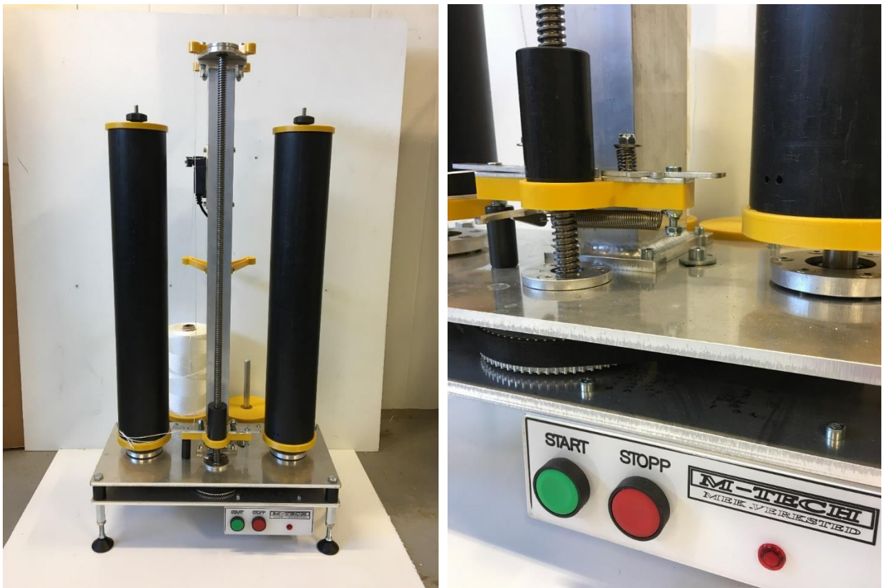
Figure 1: Device for automated spinning of twine onto spools.
