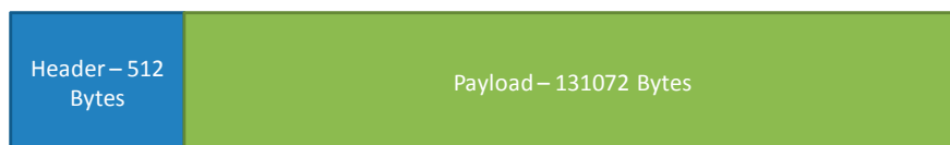
Figure 3. FITWD data packet diagram. Secondary sensor data was carried in the header.
