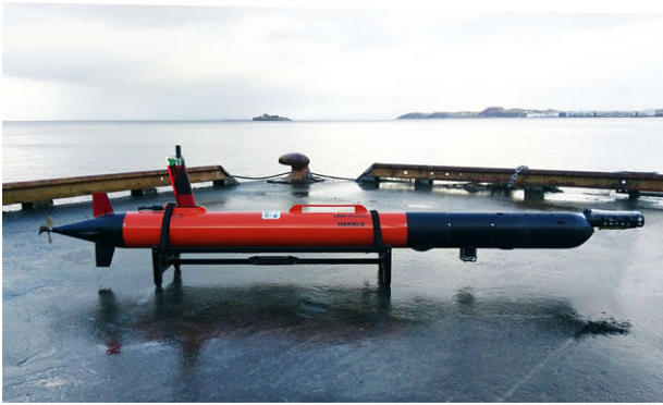
FIGURE 11 NTNU's light AUV platform ( Harald ) for upper water-column exploration used in our work—the CTD is visible in the nose. The AUV has an excess of 24 hr in-water operational capacity with a range of sensors in addition to the CTD
