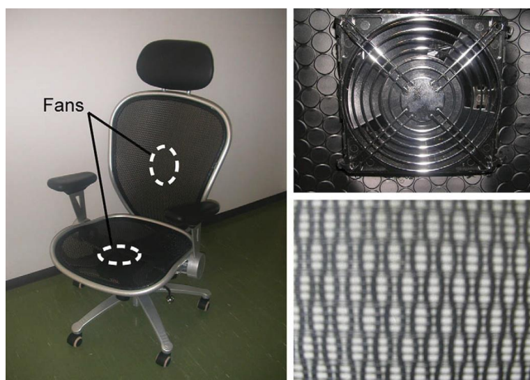
Figure 18 Left: Test chair with fans installed under the seat and behind the backrest. Right: Fan and open fabric of the chair. (Watanabe, Shimomura, and Miyazaki 2009: page 1394)
