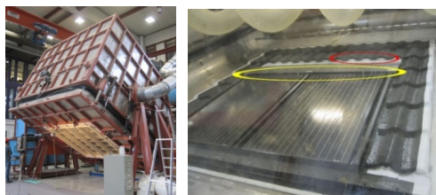
Figure 7. Large-scale laboratory investigations of wind-driven rain exposure of a BIPV system [42].
