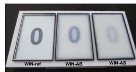
Figure 3. Photo of float glass window panes with (left) air, (middle) large-sized aerogel granulates and (right) small-sized aerogel granulates in the cavities [23].
