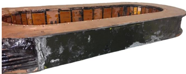
Fig. 6. Outer surface of straight section of the coil made flat to distribute the mechanical forces.
