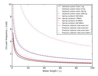
Figure 2: Natural circular frequency of the wave energy converter as function of water column length l', hydraulic piston mass  $m_{pist}$ , restoring spring stiffness  $k_{pist}$  and pressure collector inlet area A.
