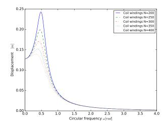
Figure 3: Maximum displacement range of the hydraulic piston.
