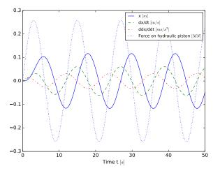
Figure 6: Numerical calculation of piston motion using an Euler model.
