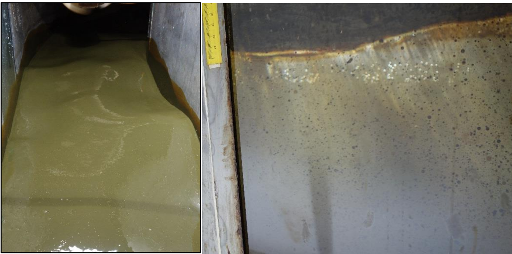
P0 – Application of Brasse in the meso-scale flume. Large oil droplets were observed in the water column
