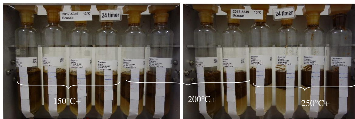
Figure 2-4: Rotating cylinders of water-in-oil (w/o) emulsions of Brasse crude oil after 24 hours at 13 °C
