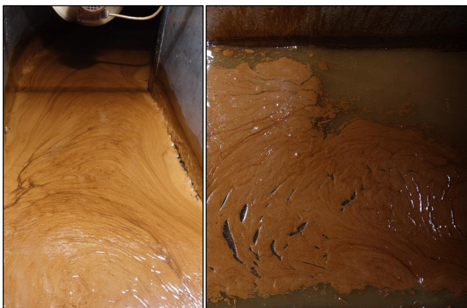
120 minutes after third dispersant application. The slick started to re-emulsify. Viscosity: 3631 mPa.s
