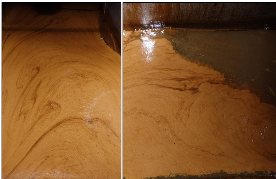
Figure 3-7: 2 nd dispersant (Dasic NS) application on Brasse
