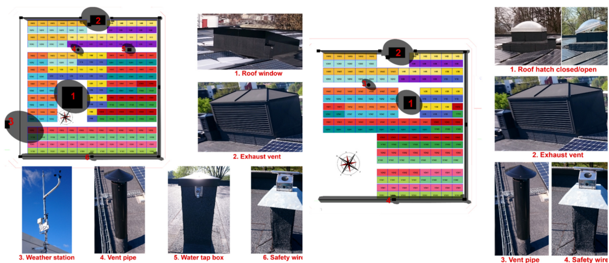
Figure 4.16 Identification of cast shadows at Block 4 (left) and Block 5 (right). (Drawing from Entra, Asplan Viak, photos by L. Ødegården) (Ødegården, 2016)
