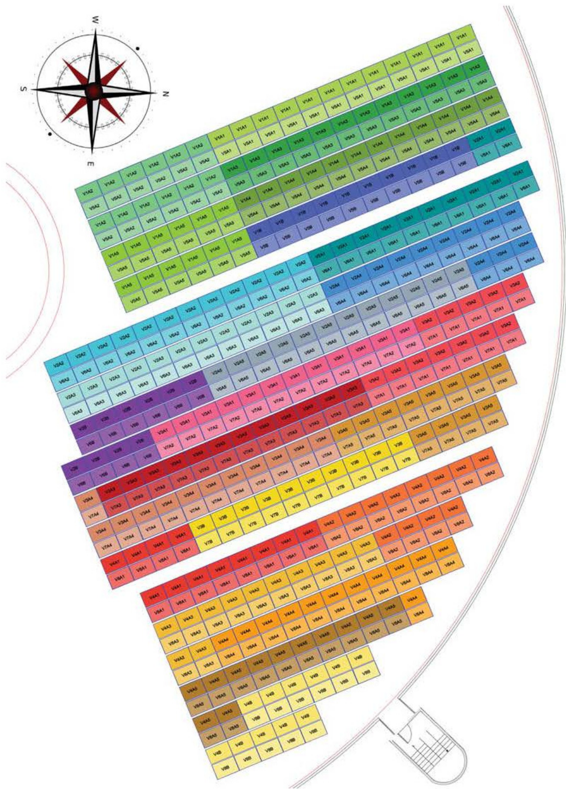
Figure A.3: Illustration showing the string configuration at the garage building. (Source: Asplan Viak, Skanska)
