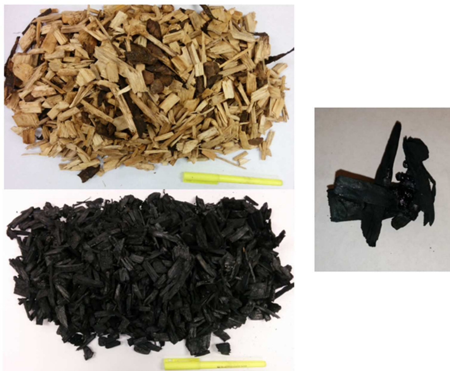
48 Figure 3: Spruce wood feed, spruce wood charcoal on the bottom and a fused particle 49 originating from experiment 4 in Table 2.
