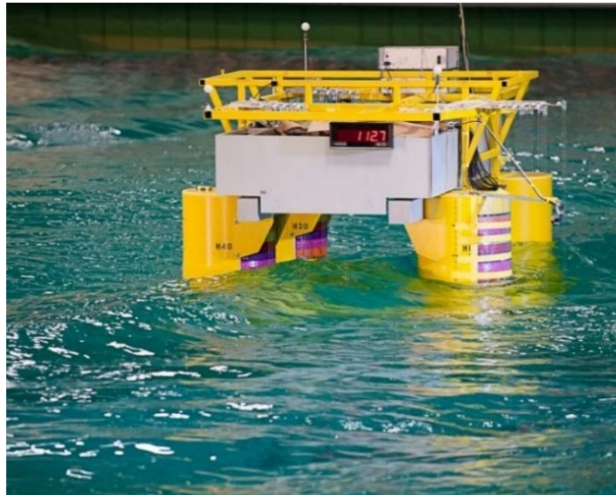
Figure 1 Heidrun model in basin (Photo: Marintek)
