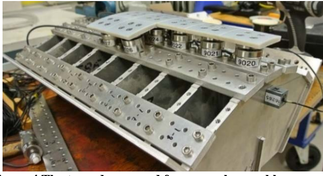
Figure 4 The transducers and force panel assembly were mounted on a stiff steel sector. (Photo: Marintek)
