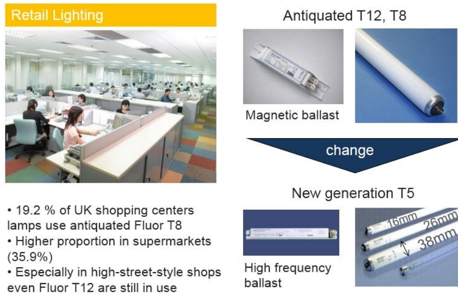
Figure 47 – Consider replacing T12 and T8 fluorescent lamps with new T5 fittings, lamps and ballast
