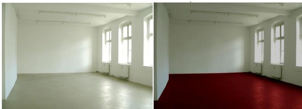
Figure 42 – Room efficiency: Different reflectivity grades for floors lead to a 50% reduction in necessary electrical wattage
