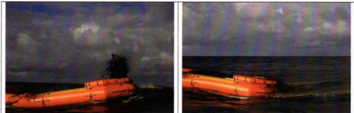
Figure 3.15. “Splash-over” of emulsion from the separator chamber of the Ocean Buster system (NOFO OoW exercise in 2008) operating “up-wind” at 2.5 – 3 m significant wave heights. Picture to right is taken just after the picture to left, showing that the emulsion “rained” on the sea-surface behind the OB-system.
