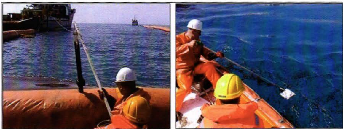
Figure 3.9. Left: Measuring of oil thickness inside the boom systems, method: cylinder apparatus. Right: Measuring of oil leakage behind the boom system using oil adsorption pads to measure film thickness.
