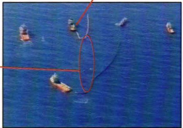
Figure 3.12: Towing speed: approx. 0.8 - 1 knot. “Significant” boom leakage.
