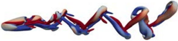
Figure 6: Vortical structure for a cylinder tilted with an angle \theta = 75^\circ at Re = 200 . Isosurface of Q = 10^{-2} coloured by the longitudinal vorticity ranging from -0.2 to 0.2 .
