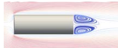
Figure 3: Standing eddy behind a L/D = 3 cylinder at Re = 200 . Instantaneous streamlines on the y - z plane are coloured by the axial velocity.
