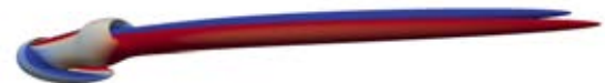
Figure 4: Vortical structure for a cylinder tilted with an angle \theta = 15^\circ at Re = 200 . Isosurface of Q = 10^{-2} coloured by the longitudinal vorticity ranging from -0.2 to 0.2 .
