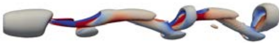
Figure 2: Wake patterns of a L/D = 1 cylinder aligned with the streamwise direction at Re = 360 . 96 cells are distributed along the cylinder diameter. The wake is visualized using the Q criterion. Isosurface of Q = 10^{-3} are shown. Those isosurfaces are coloured by the horizontal vorticity ranging from -0.2 to 0.2 .
