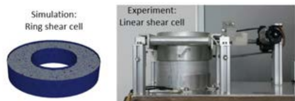
Figure 5: Calibrating the particle-particle coefficient of friction with shear cell experiments and simulations.
