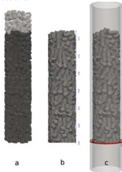
Figure 1: Packing creation for mono-disperse cylinders: a – filling the beds with DEM code, b – correcting the bed heights to 0.013 m and exporting the STL, c – merging the main bed and particles STLs.
