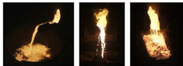
Figure 1: Tapping in operation on a DC furnace pilot plant, (l) and (m) slag, (r) metal (images courtesy Mintek)
