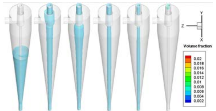
Figure 8: Iso surface for contour level 0.005 volume fraction for phases left to right: phase 6 to phase 1
