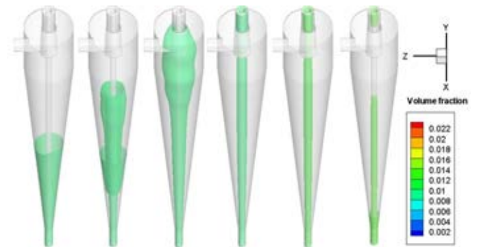
Figure 9: Iso surface for contour level 0.01 volume fraction for phases left to right: phase 6 to phase 1
