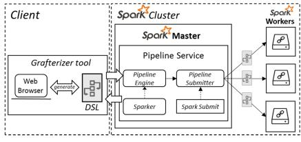
Fig. 2. High-level architecture of the service
