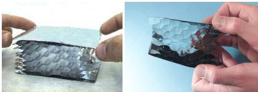
Fig.20. View of the barrier foil and the baffle structure inside a gas-filled insulation panel ( http://gfp.lbl.gov/ ).
