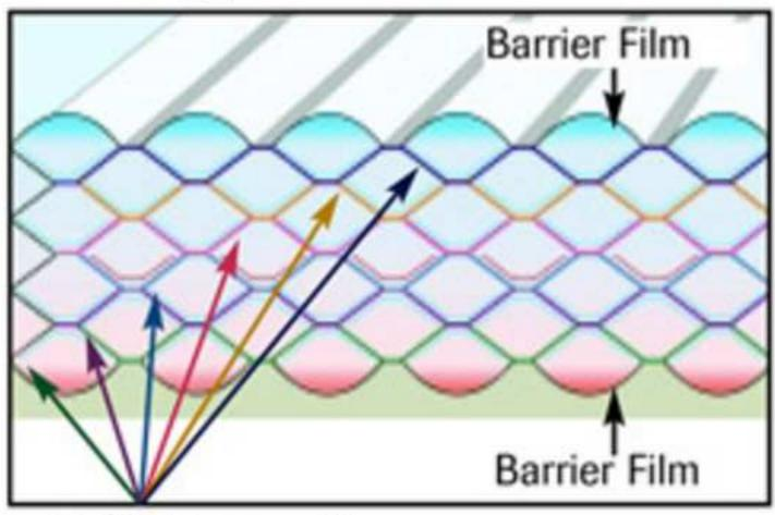
Baffled low emittance polymer chambers Fig15-Left Click here to download high resolution image
