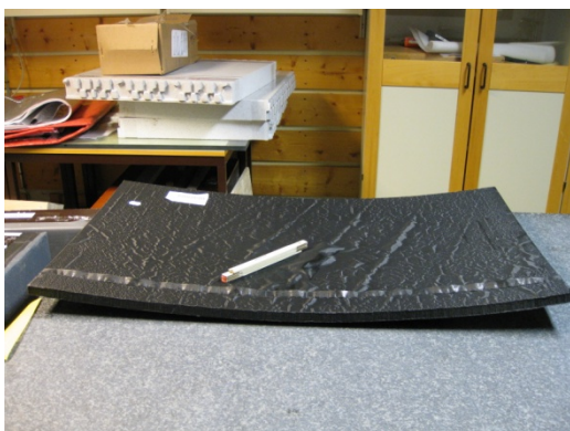
Fig. 20 Exposed panel after exposure to cyclic climate strains in vertical climate simulator for approximately one month. Some delamination of the fleece cover is visible. The panel had curved during exposure. No further changes were observed during the rest of the ageing period.
