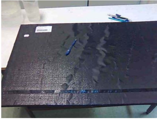
Fig. 17 Visible delamination of the outer fleece layer of the VIP envelope after exposure at 80°C for 7 days.
