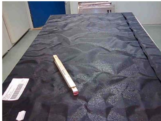
Fig. 18 Visible delamination of the fleece cover after exposure at 80°C for approximately 1 month. More of the envelope cover has lifted from the substrate than after 7 days. No further changes were observed during the rest of the ageing period.
