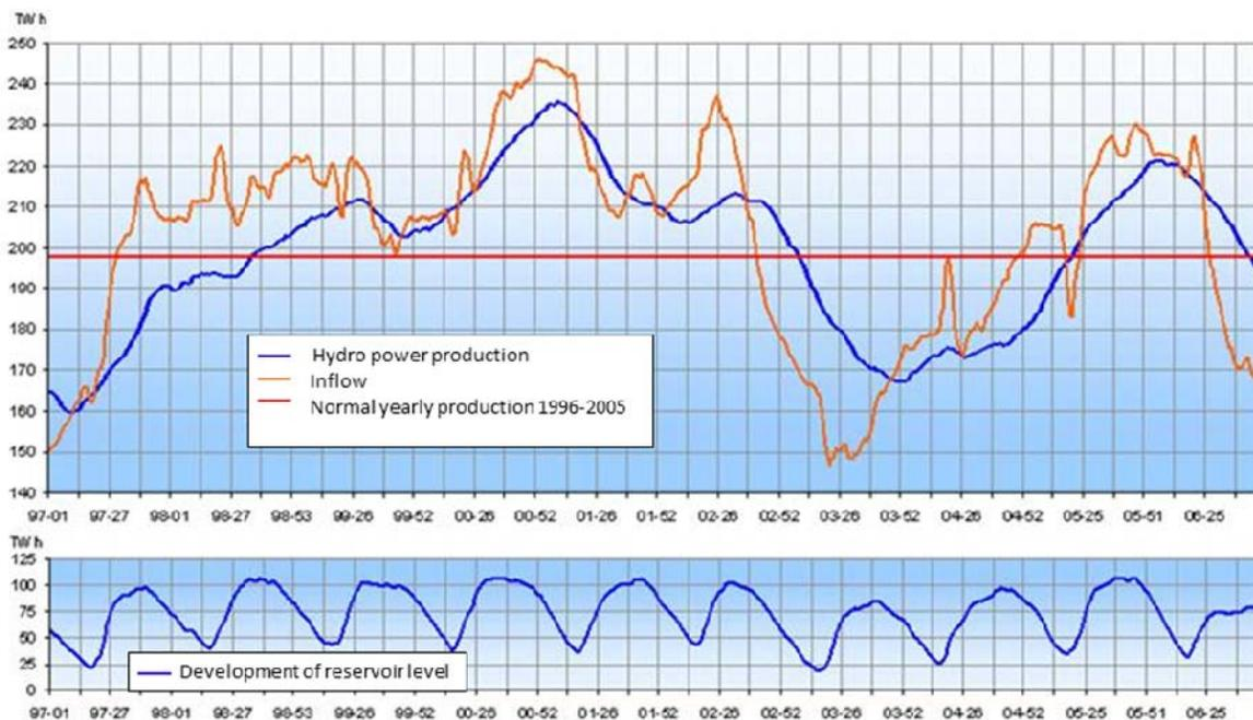
**Figure 15 Inflow, hydro power production and development of reservoir levels in Sweden from 1997-2006 [19]**
