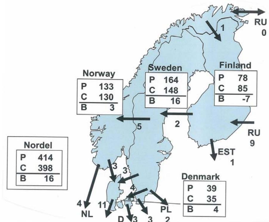
Figure 2 Expected electricity balance in 2012 (TWh) [7]. P=Production, C=Consumption, B=Balance without energy exchange. The estimations consider an average inflow.
