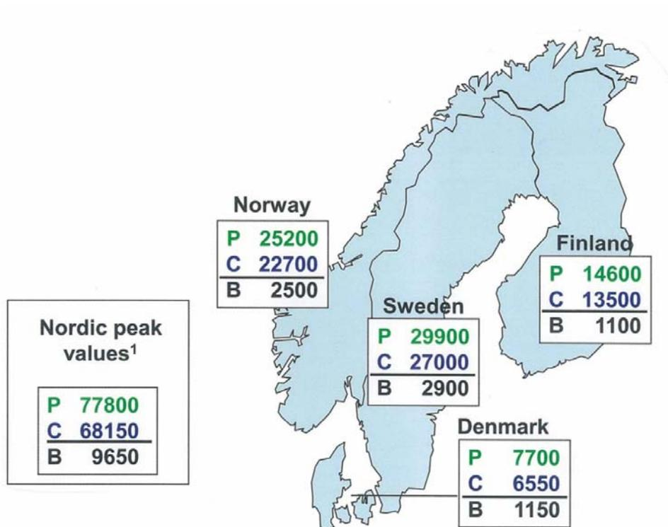
**Figure 3 Expected available power capacity and peak demand 2012/13 (MW) [7]. P=Production, C=Consumption, B=Balance without energy exchange.**
