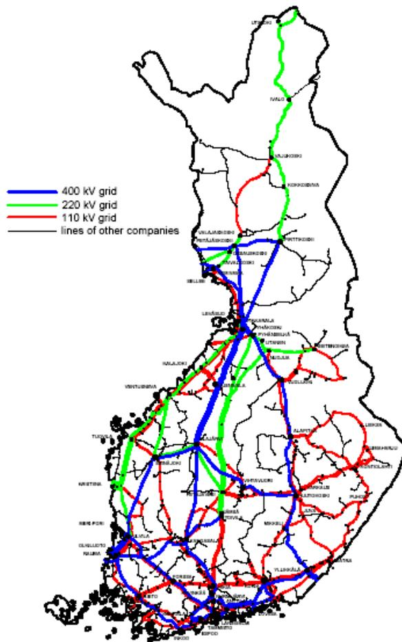
Figure 18 Finland's High Voltage Electricity Grid (as of December 2001) [22]
