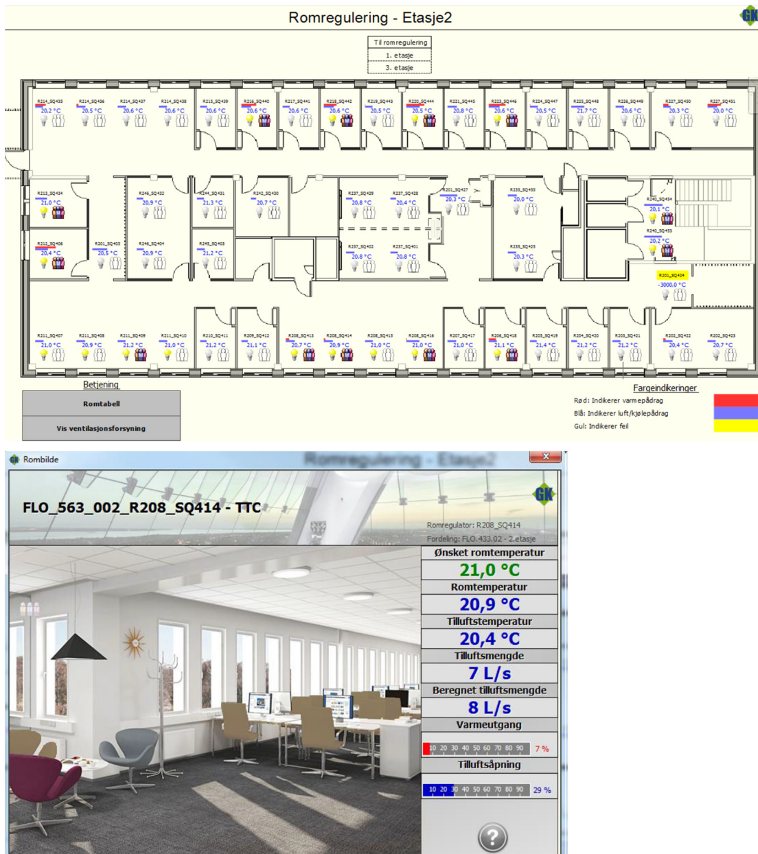
Figure 4.5 Room system with clickable floor- and room-interface that enables easy set-point adjustments and default detection.
