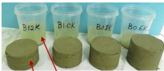
Filter cake and passed material (mainly water) for cement B, filter size=75 \mu m
