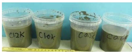
Grout passed through the filter, cement C at 8° C filter size=75 \mu m
