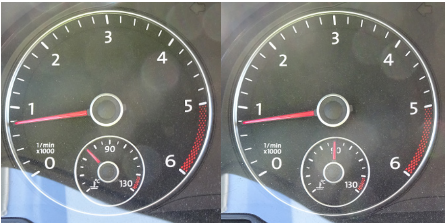
Figure 34: Oil temperature of VW Caddy. Right: 70 °C (start of test), Left: 90 °C (normal temp.)
