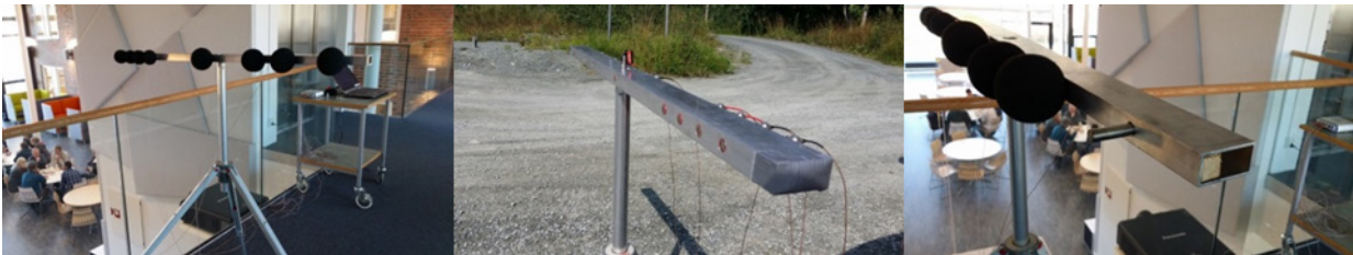
Figure 8: Microphone array used for test
