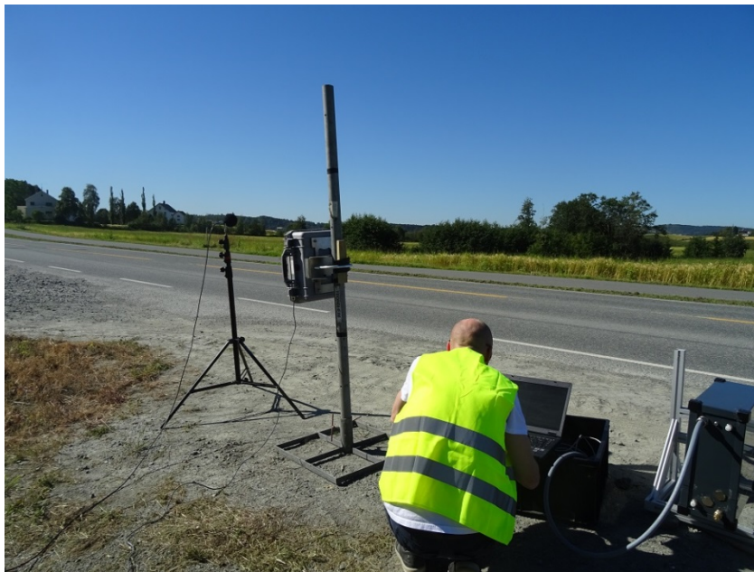
Figure 33: TOPO-bigbox and microphone set-up at Bratsbergveien
