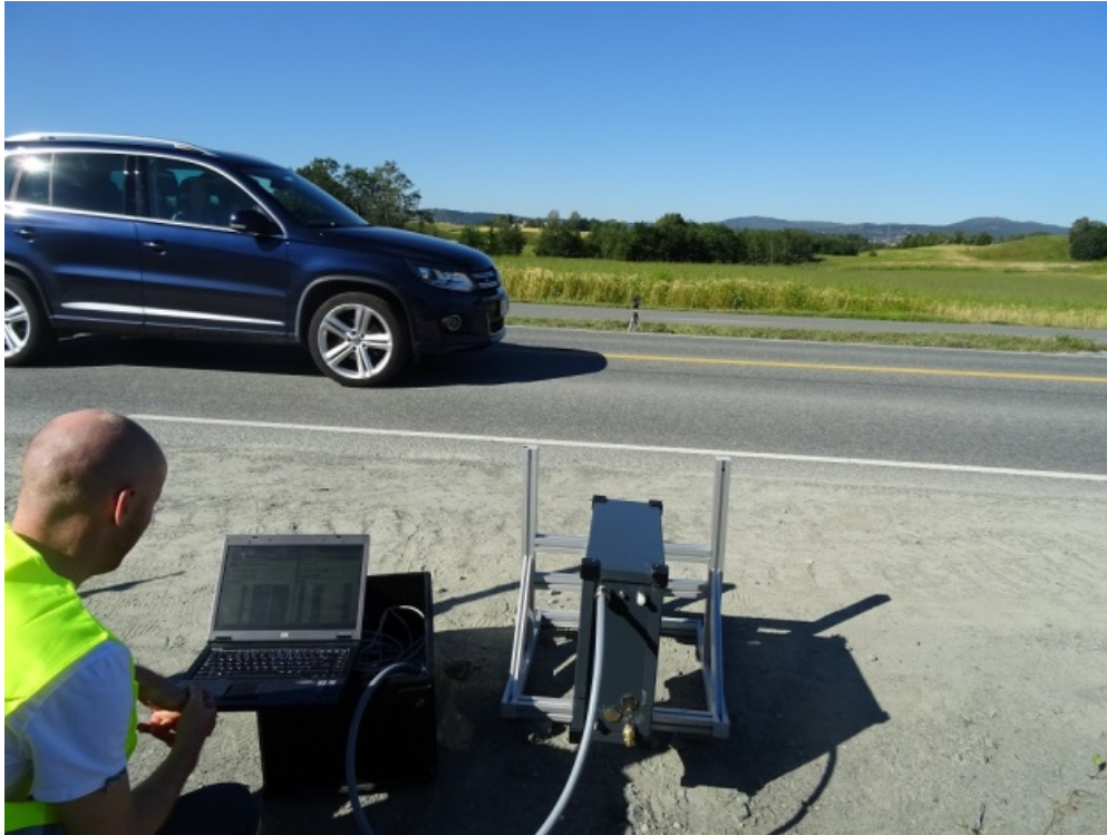
Figure 32: Set up with LaserGas iQ 2 , with reflector on the opposite side of Bratsbergveien
