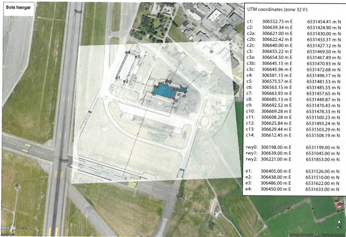
Figure 1: Image overlay of hangar buildings in Google Earth . UTM coordinates of the buildings are thereafter found. Notice that a certain level of image transparency is necessary to get a good enough match between the overlay image and the Google Earth image. Notice also that the centerlines of the runways are marked for the case of the subsequent analysis.
