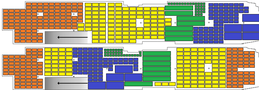
Fig. 1: Two different stowage plans for a given deck and cargo list. The exit ramp is marked with an arrow. Each colored square represents a vehicle and all vehicles with the same color are unloaded at the same port. Unloading sequence: Blue, green, yellow, orange. Thus, the blue vehicles are unloaded at the first unloading port and the orange ones at the last port on the voyage.
