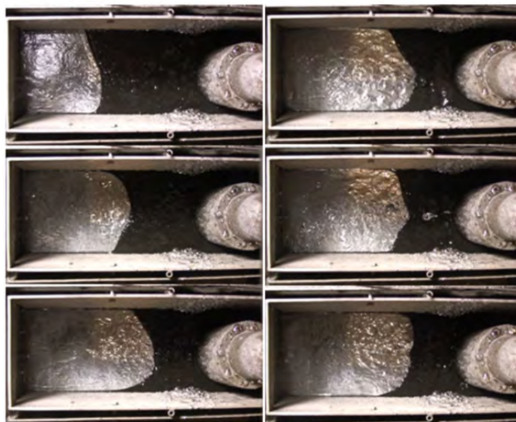
Figure 12: Video snapshots of the metal slag interface during argon injection tests at CCS-1 (taken every 10 seconds for a total time of 1 minute) for an argon mass flow rate=4 lt/min.
