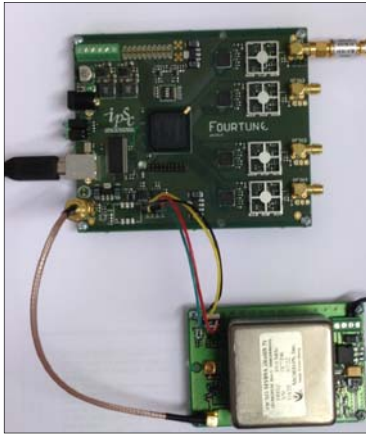
Figure 5. Fourtune receiver board outside of enclosure casing showing connection to VC-OCXO oscillator. In the deployed configuration each of the four independent RF channels are connected to a common RF feed from the GNSS antenna.
