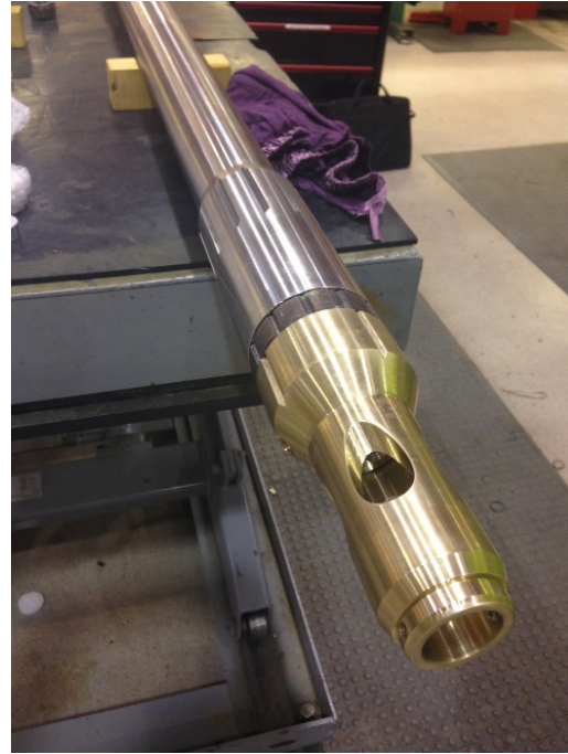
Figure 1. Pressure housing which encapsulates the heat shield. A nose protector protects the temperature sensor and the pressure port.
