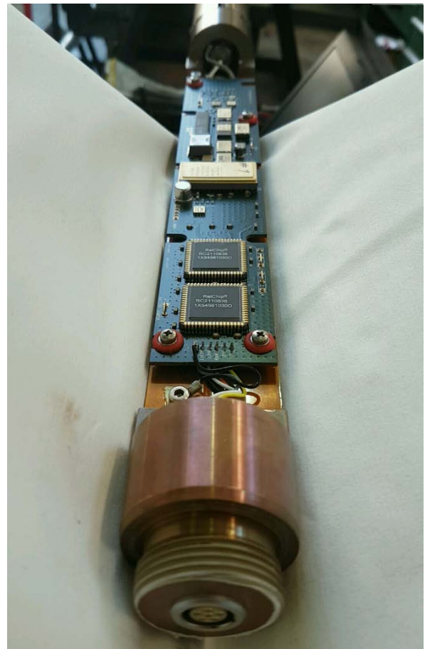
Figure 4. Picture shows assembled PCB mounted in the electronic slot of the heat sink.
