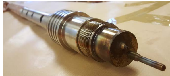
Figure 2, Pressure port and temperature sensor in the nose of the tool. Pressure and heat shield, and nose protector, are removed.
