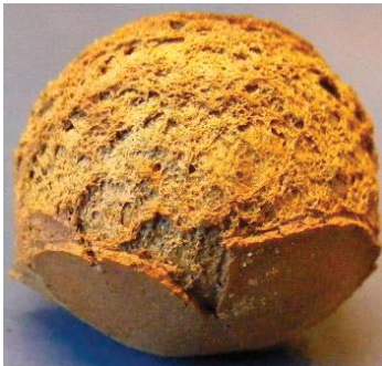
66 67 68 69 70 71 72 73 74 75 76 77 78 79 80 81 82 83 84 85 86 87 88 89 90 91 92 93 94 95 Caption Fig. 3: Illustration of one pellet of the series lab-16 (16 mm diameter) picturing the heterogeneity of the outer shell. The lower hemisphere exhibits a dense shell; the upper hemisphere exhibits a more porous shell.
