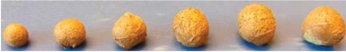
11 12 13 14 15 16 Caption Fig. 2: Illustration of LWA pellets produced in a chamber furnace in the laboratory.
