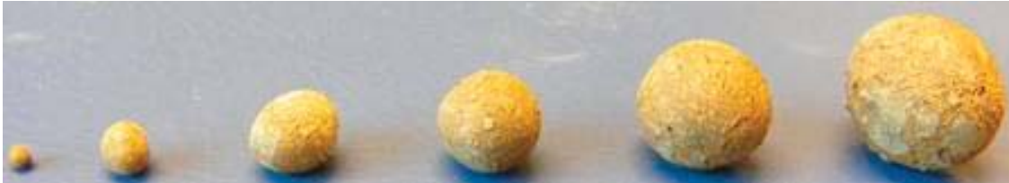
Caption Fig 3: Illustration of the reference material produced in a pilot-scale rotary kiln.
