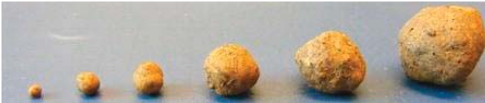
Caption Fig. 4: Illustration of carbon steel fibre containing LWA produced in a pilot-scale rotary kiln. Diameters range from 1.8 mm (left) up to 12 mm (right).
