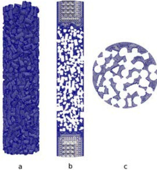
Figure 2: Mesh created for mono-disperse cylinders: a – mesh on the particles surfaces, b – mesh on the vertical centre cut plane, c – mesh on the horizontal centre cut plane.
