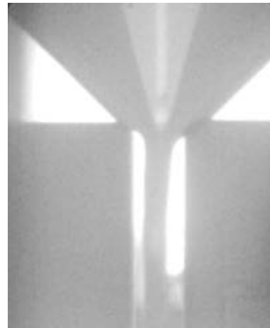
Figure 7: Gas distribution in the upper part of the SEN. Experiments at X-LIMMCAST with a liquid flow rate of 140 \text{ cm}^3/\text{s} and a gas flow rate of 1.7 \text{ cm}^3/\text{s} .
