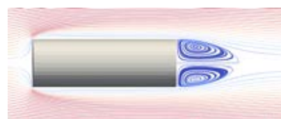
Figure 3: Standing eddy behind a L/D = 3 cylinder at Re = 200 . Instantaneous streamlines on the y-z plane are coloured by the axial velocity.
