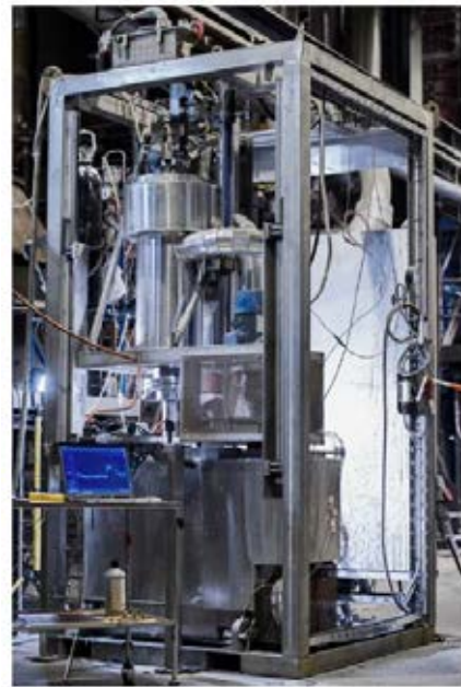
Figure 3: CCS-1.5 Continuous Casting SimulatorThe CC simulator was used to test two different SEN types; namely mountain and cup, based on the shape of the bottom of the nozzle and ports (Figure 4). The mountain and cup types are designated M and C, respectively.
