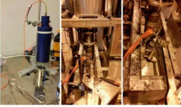
Figure 5: Measurement of fluctuations at the metal interface using an optical probe.
