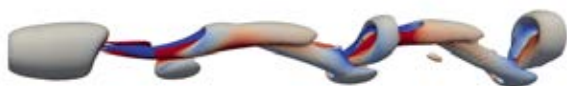
Figure 2: Wake patterns of a L/D = 1 cylinder aligned with the streamwise direction at Re = 360 . 96 cells are distributed along the cylinder diameter. The wake is visualized using the Q criterion. Isosurface of Q = 10^{-3} are shown. Those isosurfaces are coloured by the horizontal vorticity ranging from -0.2 to 0.2 .
