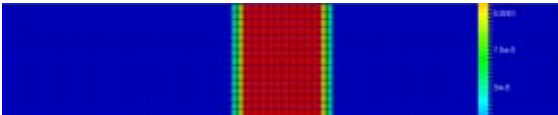
Figure 3: The sulfur mass fraction presenting a discontinuity (the filler metal) at t = 0 s, x = 0 cut.
