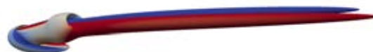
Figure 4: Vortical structure for a cylinder tilted with an angle \theta = 15^\circ at Re = 200 . Isosurface of Q = 10^{-2} coloured by the longitudinal vorticity ranging from -0.2 to 0.2 .
