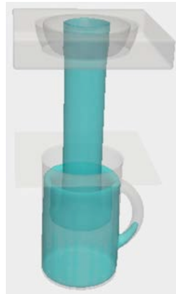
Figure 3: Container filling with complex geometry. Simulation on 8 cores.
