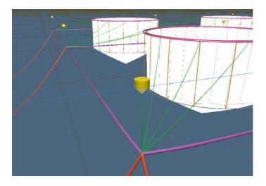
Figure 3: Aquaculture site modelled by separate model components. Cable widths exaggerated for visibility and connection plates are not shown.
