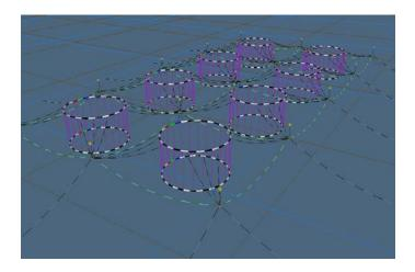
Figure 5: Visualization of the developed model of an aquaculture site. All structure elements reside in the same model and allows the model to have good performance even with a high level of interconnected flexible elements.
