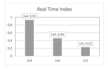
Figure 6: Real time performance of site model vs number of cells in model.
