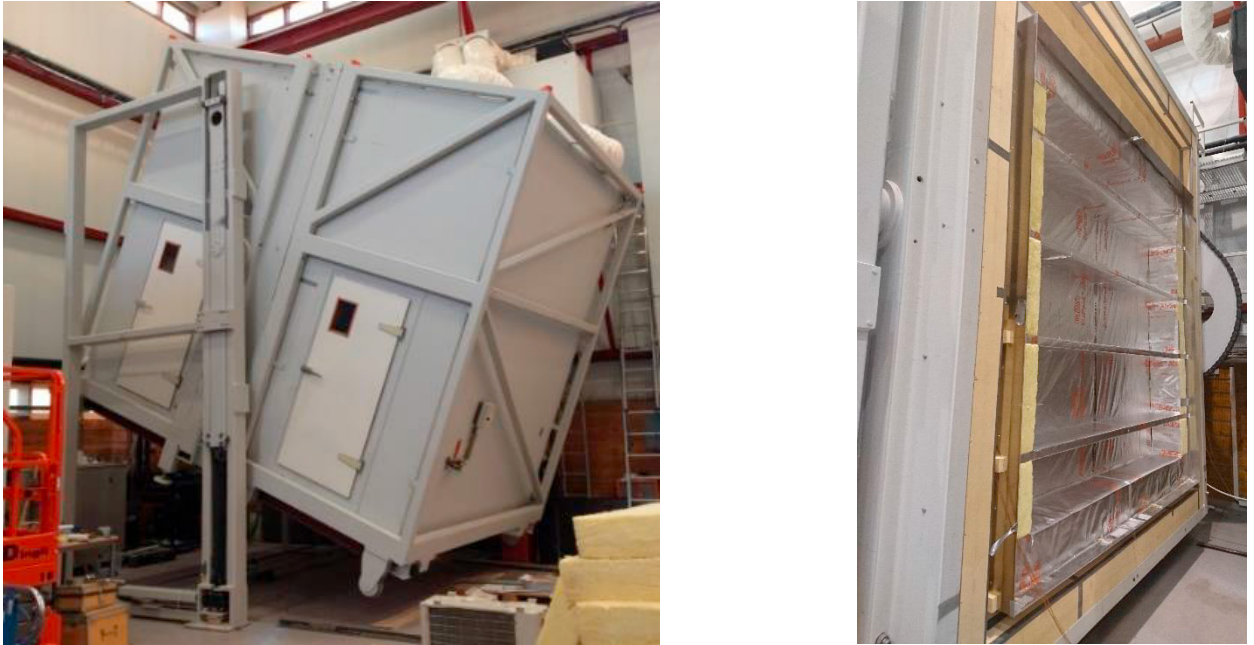
Fig. 2. Photo showing the pivotal hot-box (left). The test floor specimen was mounted between the cold room and the metering chamber/guard room and was in horizontal position during the tests. The timber frame test section variant V7 under rebuilding (right).
