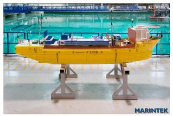
Figure 1: EXWAVE FPSO 1:70 scaled model.
