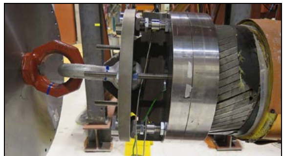
FIGURE 8. END OF TEST SAMPLE WITH SIMPLIFIED END FITTING AND LINER FORCE MEASUREMENT SYSTEM INSTALLED
