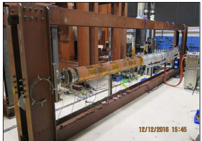
FIGURE 9. TEST RIG WITH PIPE SAMPLE INSTALLED. INSULATION IS REMOVED FOR VISUALIZATION
