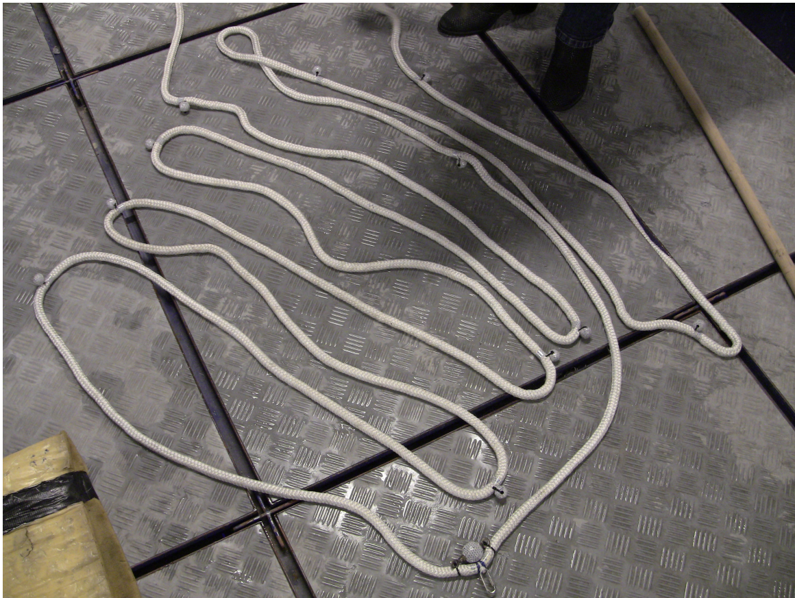
Figure 15: The combination rope laid out on the platform of the flume tank. Showing the very small bending stiffness
