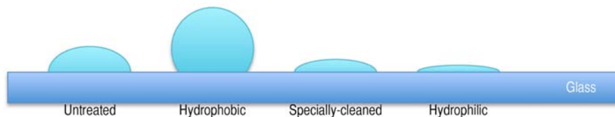
Figure 3: Illustration of a typical physical form of a water droplet on untreated, hydrophobic, specially-cleaned and hydrophilic glass. The contact angle is at maximum for a hydrophobic surface and at minimum for a hydrophilic surface, with untreated and specially-cleaned in between. Source: Redrawn illustration from figure by Ritec International [8]
