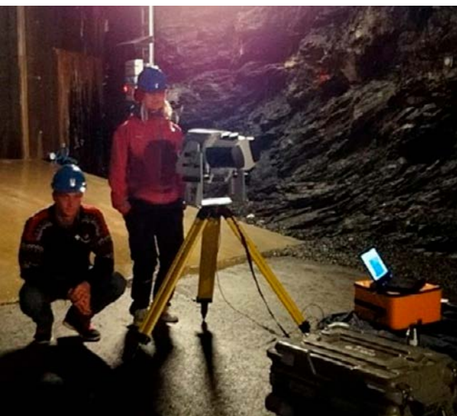
Measurement by using TLS in a hydropower tunnel.
