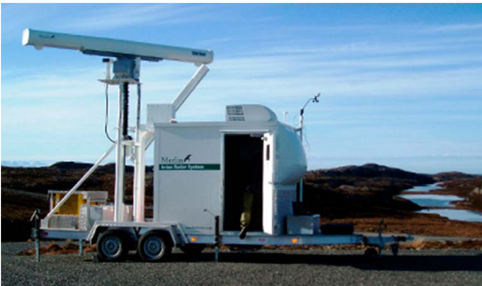
ROBIN mobile avian radar – monitoring bird movements where and when this is required. Photo: Roel May
