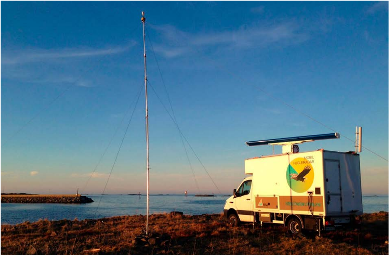
ROBIN mobile avian radar – monitoring bird movements where and when this is required. Photo: Roel May
