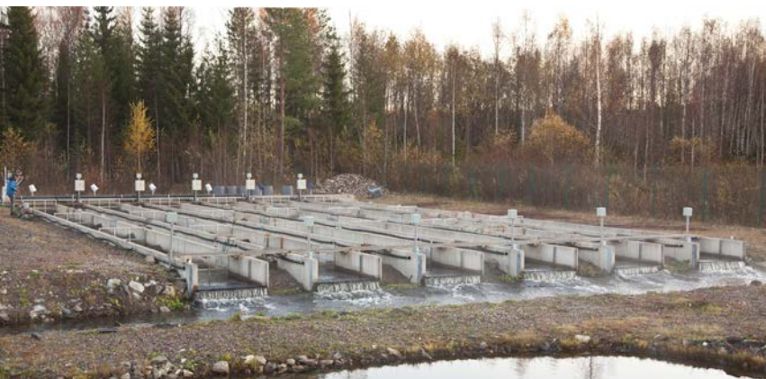
Six stream channels in Paltamo, Finland was an important arena for Michael Puffer when he showed that daily peaking waterflow had only small effects on energy storage and growth of salmon parr. Photo: Per Harald Olsen
