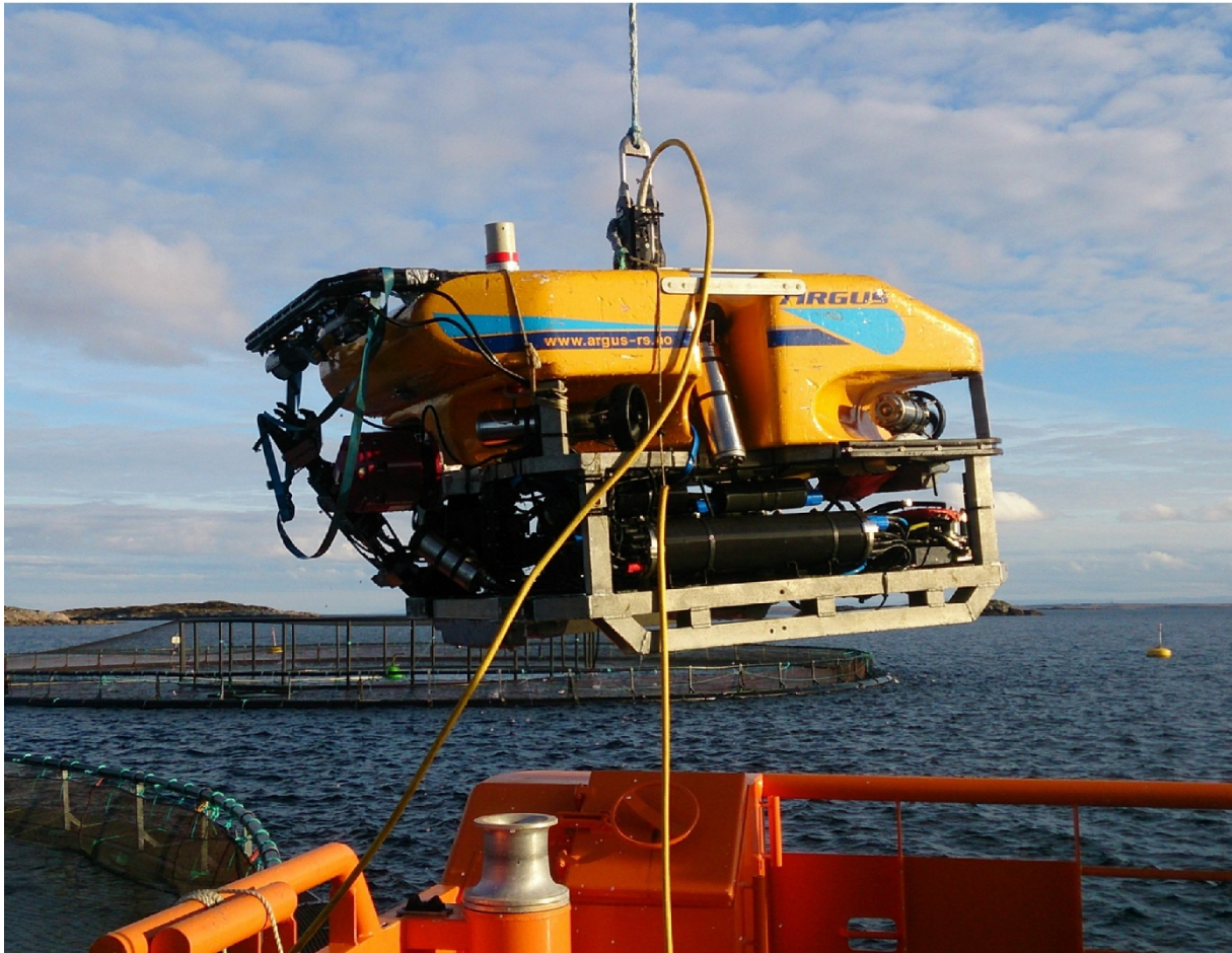
Fig. 1: Argus Mariner ROV used in the experiments, here lifted over the deck of the supplying aquaculture service vessel, which was moored to the net pen floating collar (Photo: Per Rundtop)
