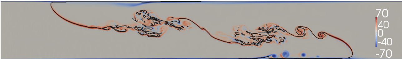
Figure 10: Numerical simulation with the present flow solver of two-phase flow. Simulation shows gravity currents obtained from a lock-exchange configuration, driven by gravity due to differences in fluid density. A breaking head-wave with droplet entrainment, as typical for contained oil of conventional oil-booms in operation, is observed.
