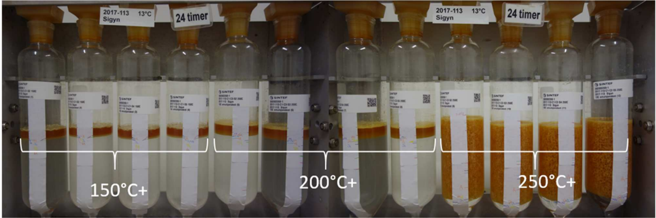
Figure 3.4 The rotating cylinders showing the emulsification of seawater in oil after 24 hours at 13 °C.
