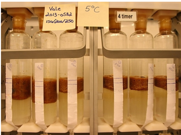
Figure 3-5: Emulsions formed after 4 hours at winter temperature (5°C).
