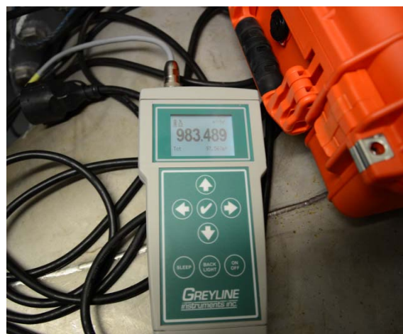
Figur 6-4: Greyline PDFM 5.0 enheten under pumping viser strømnig i m 3 /time.
